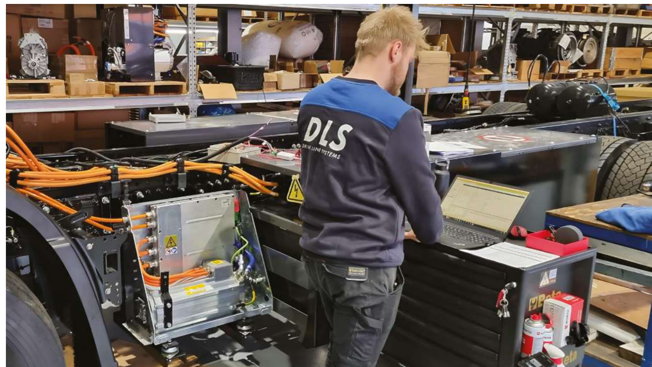
Commissioning of an electric PTO
